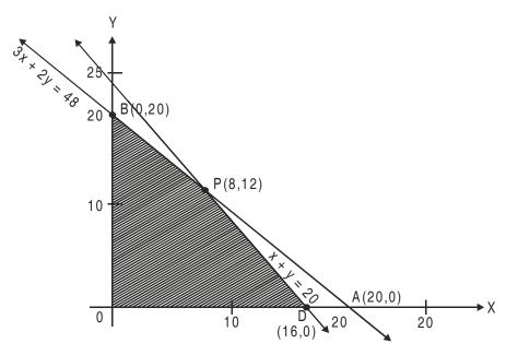
The feasible region ODPB of the L.P.P. is the shaded region which has the corners O (0, 0), D (16, 0), P (8, 12) and B (90, 20)
